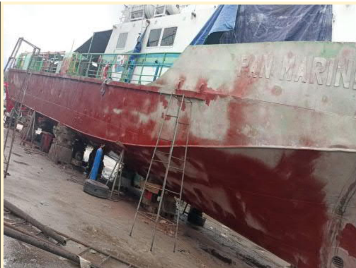
Touch up coat Intertuf 262 (KHA303/A062) red at Topside & Underwater area
