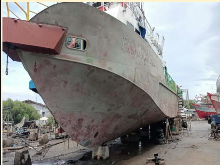
Sweep & spot blast at topside & underwater area
