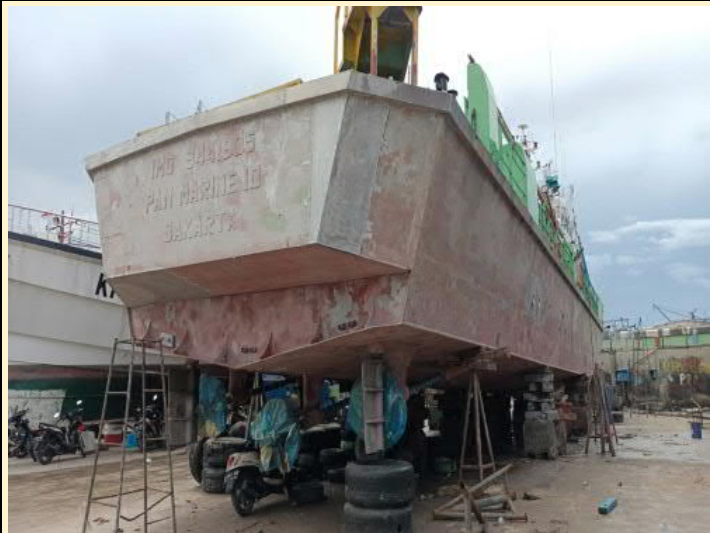
Sweep & spot blast at topside & underwater area
