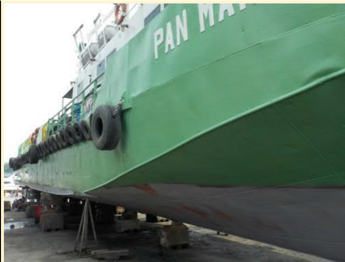
Finish coat Interthane 990 (PHF445/A) Estuary Green at topside & Touch up Intergard 263 Light grey at Underwater area
