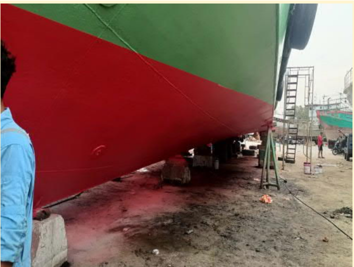
Full coat Interspeed (BQA377) red at underwater area.
