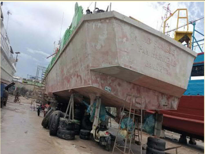
Sweep & spot blast at topside & underwater area
