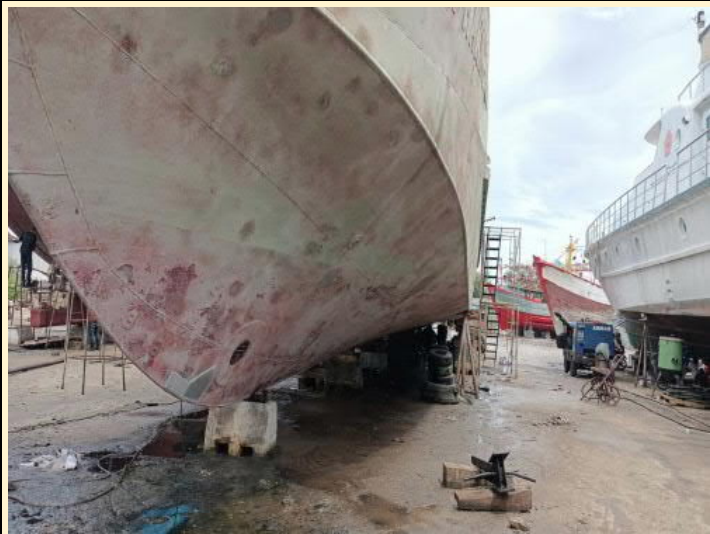
Sweep & spot blast at topside & underwater area
