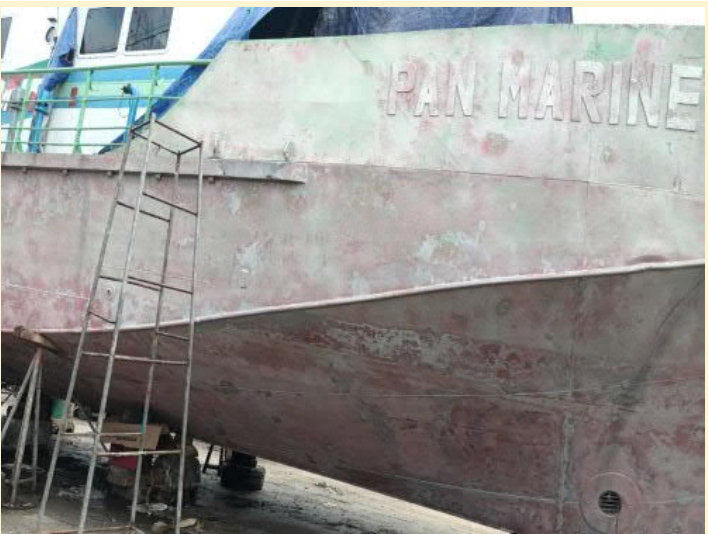
Sweep & spot blast at topside & underwater area
