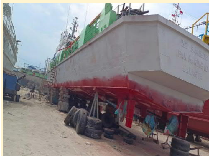
Touch up coat Intergard 263 (FAJ0034/A262) Light grey at Topside area.
