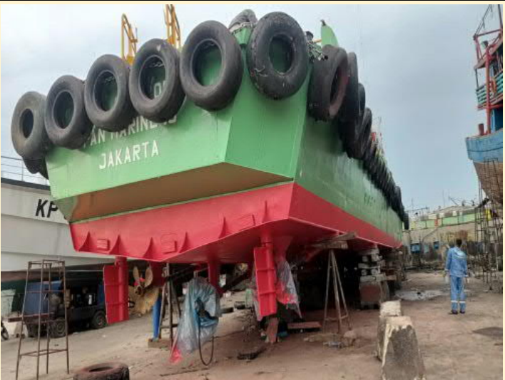
Full coat Interspeed (BQA377) red at underwater area.
