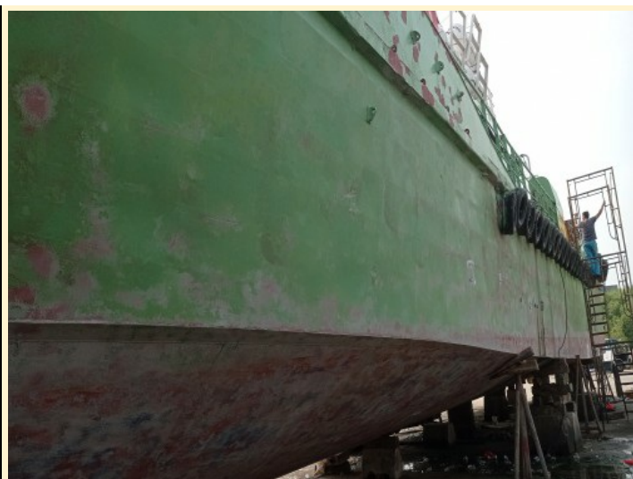
Sweepblast at topside & underwater area
