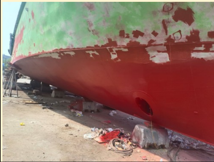
Fullcoat Intertuf 262 (KHA303/A) Red at underwater area.
