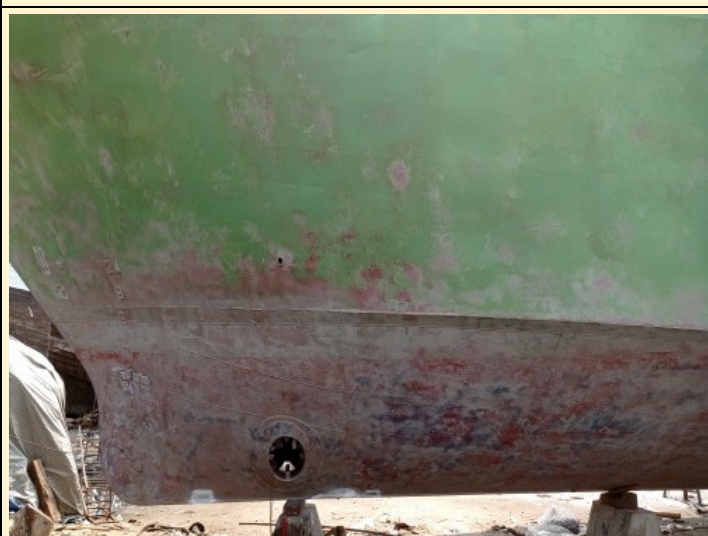
Sweepblast at topside & underwater area.
