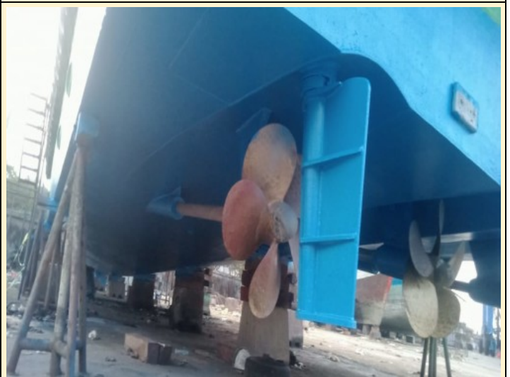
Full coat Interspeed 376 (BQA372) Blue at underwater area.
