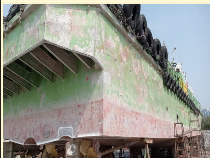
Sweepblast at topside & underwater area
