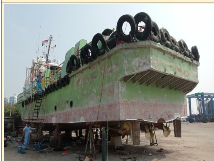
Sweepblast at topside & underwater area.
