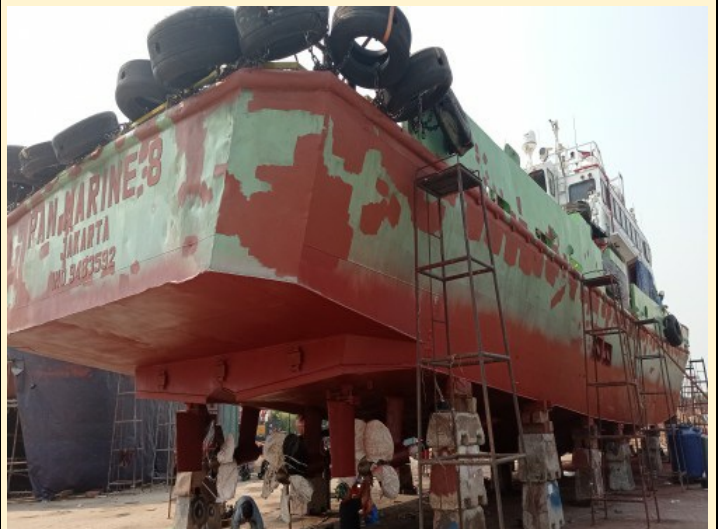
Painting 1st coat Intertuf 262 Red (KHA303/KHA062) in underwater area.
