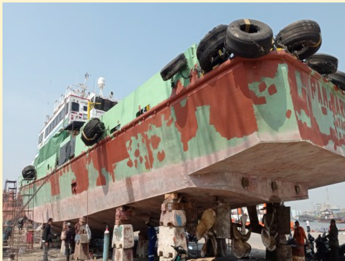
Showing result sweepblast on underwater area.
