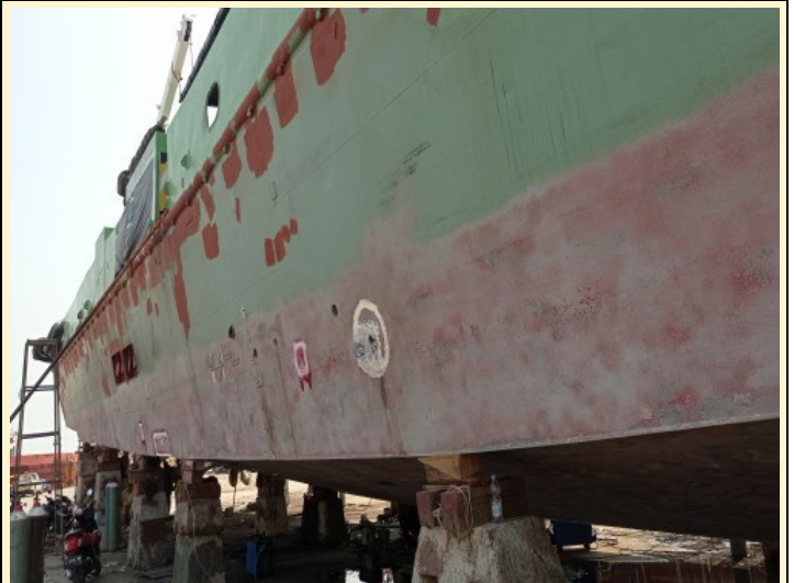
Showing result sweepblast on underwater area.
