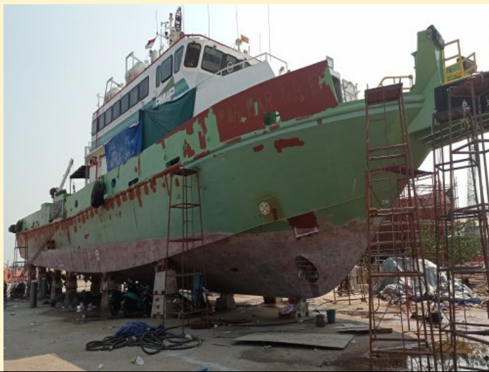
Showing result sweepblast on underwater area.
