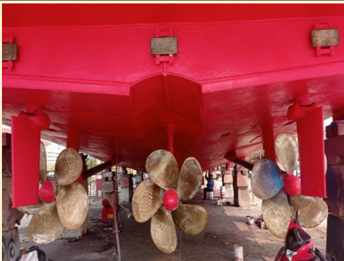
Painting 4th coat Interspeed 376 Red (BQA377) in underwater area.
