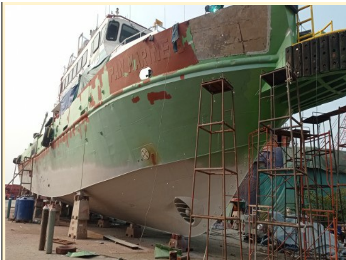
Painting 2nd coat Intergard 263 Light grey (FAJ034/FAA262) in underwater area.
